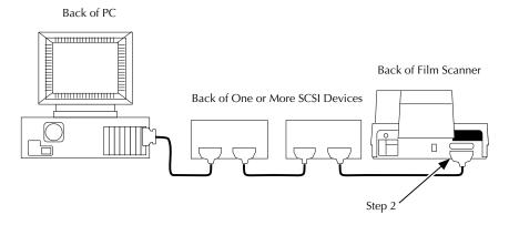
3. Attach the SCSI terminator (supplied with the Scanner) to the empty SCSI port on the Scanner, seat the terminator firmly, and pinch the wire clamps shut.
